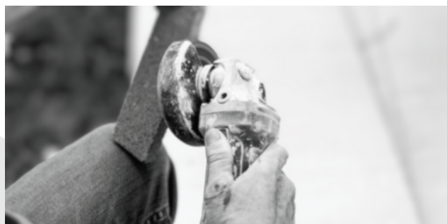
Angle grinder may also be used for cutting BioBasedTiles®.
