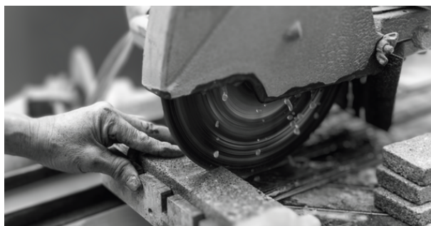
Wet saw required for cutting BioBasedTiles®.
