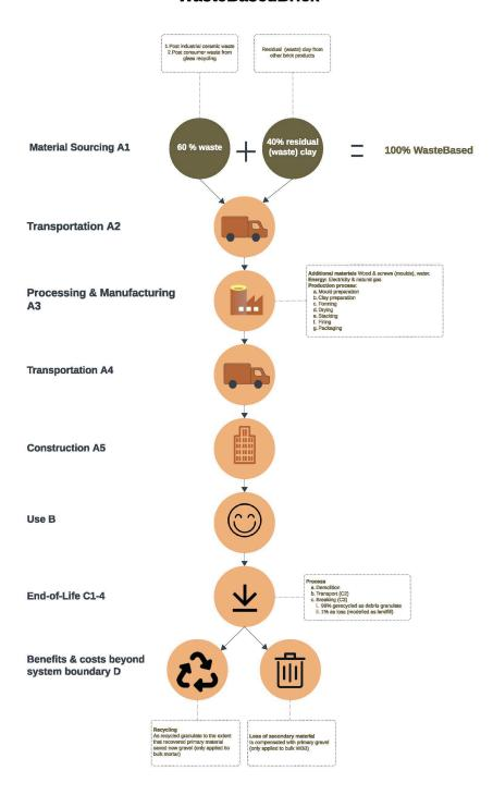
LCA process diagram according to EN 15804 (7.2.1)
