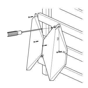
3. Begin at the left bottom corner or the middle of the bottom row. Install and screw in the bottom row, using three screws per tile.
